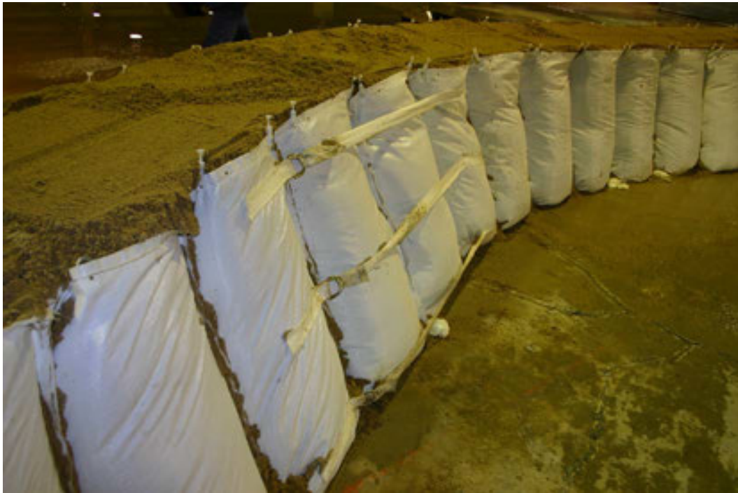
Figure 12. Straps fastened to "D" rings connect adjacent sets of bags.
