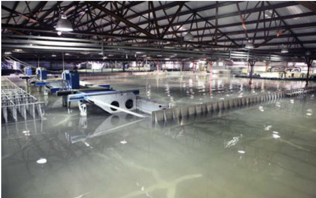
Figure 1. Research basin with wave machines on the left side and the test area on the far right. The test area is shown in closer view in Figure 2 and Figure 3.
