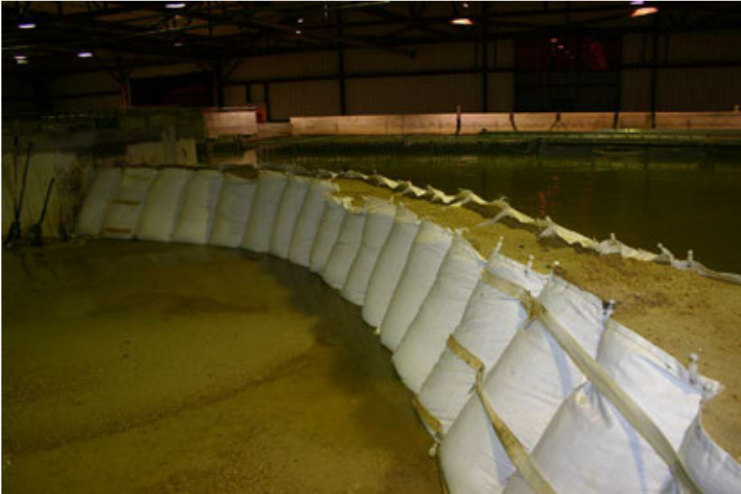
Figure 37. At the conclusion of the waves tests, looking along wall "B" towards the curve of wall "A".
