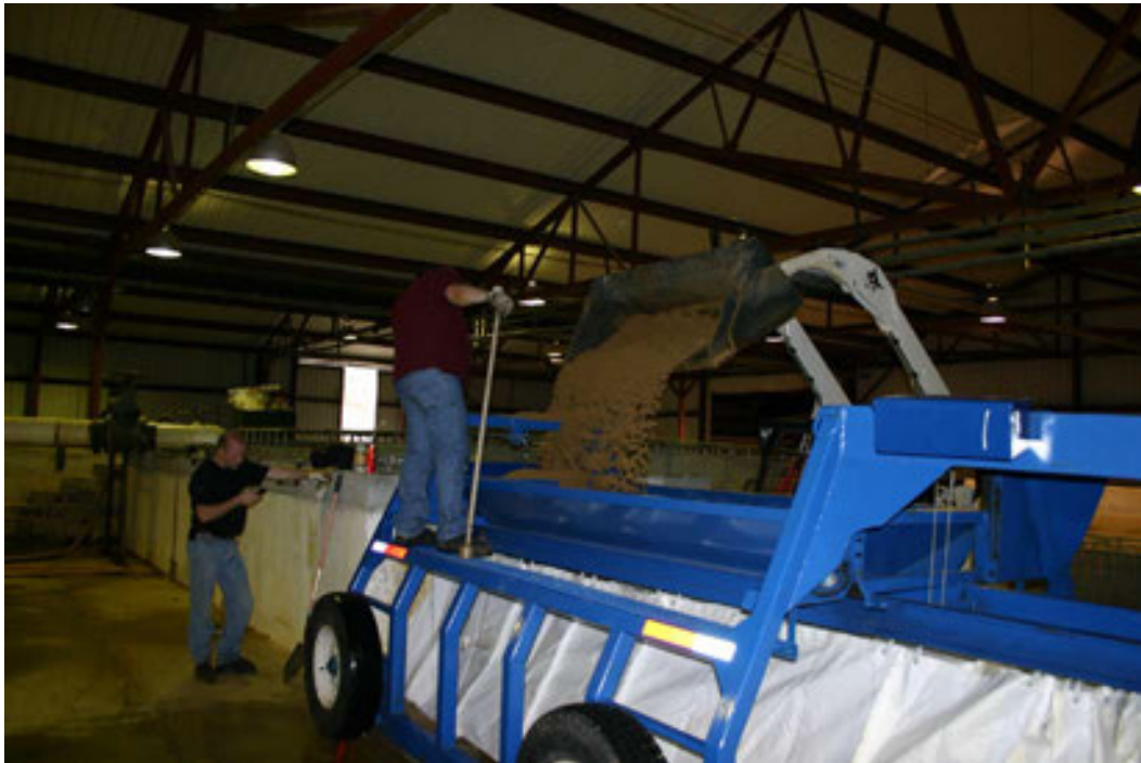
Figure 9. Sand is dumped into the hopper which holds the bags open and directs the sand into the bags.
