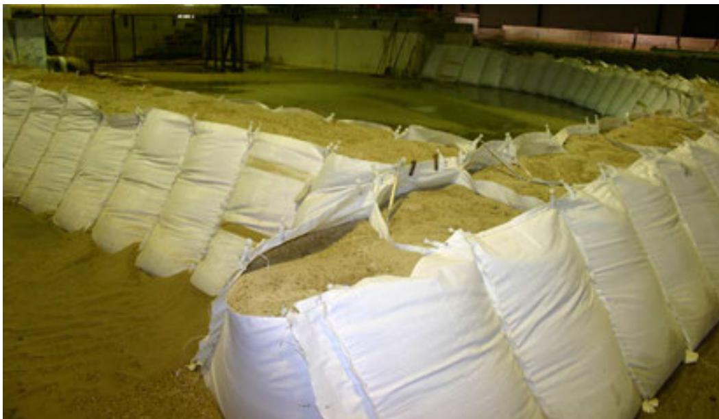
Figure 2. Test area surrounded by the RIBS flood fighting barrier at the conclusion of test protocol.
