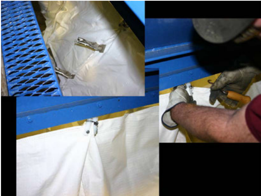
Figure 13. Baling wire around the mounting pins and vice-grip clamps hold adjacent sets of bags together.
