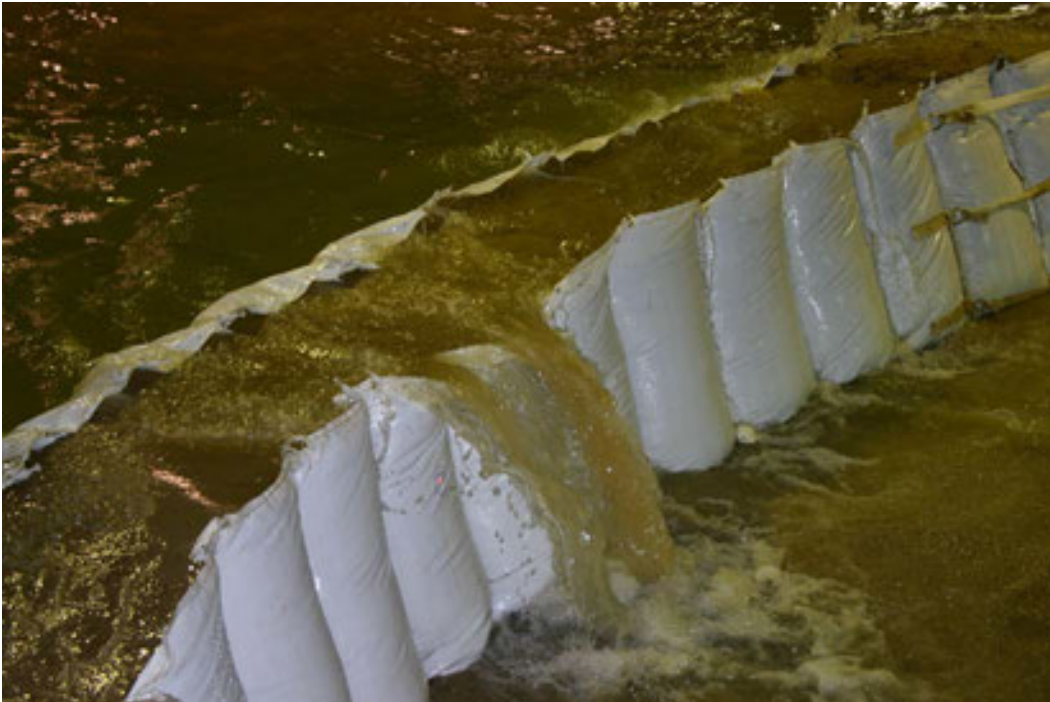
Figure 36. Wave overtopping along wall "A" during test at high water level with large waves.
