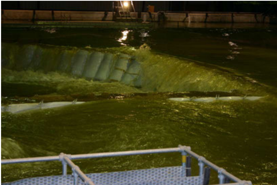
Figure 44. Large waves added to the overtopping test.
