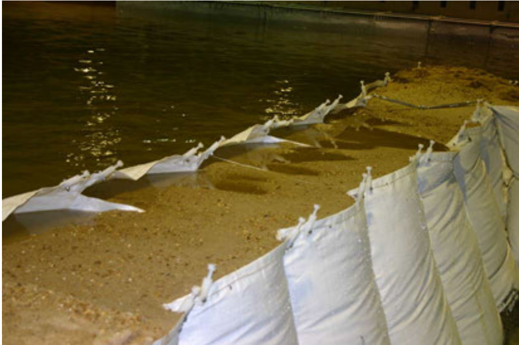
Figure 31. Washout along outer wall of wall "B" after test at low water with large waves.
