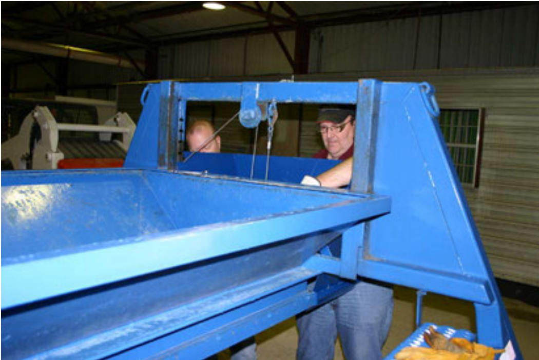
Figure 6. Hopper being lowered on deployment trailer.
