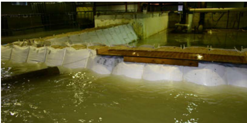
Figure 4. Test area after debris-impact test showing the sump in the back corner of the test area.
