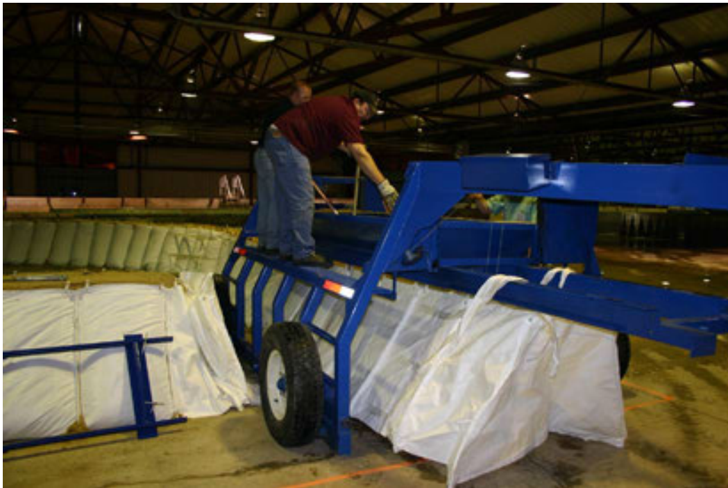
Figure 5. RIBS units being filled with sand through the hopper on the deployment trailer.
