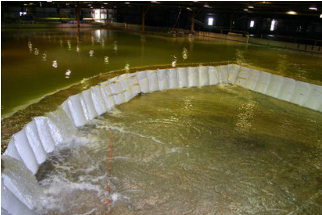
Figure 43. Water flowing over the structure during the overtopping test.
