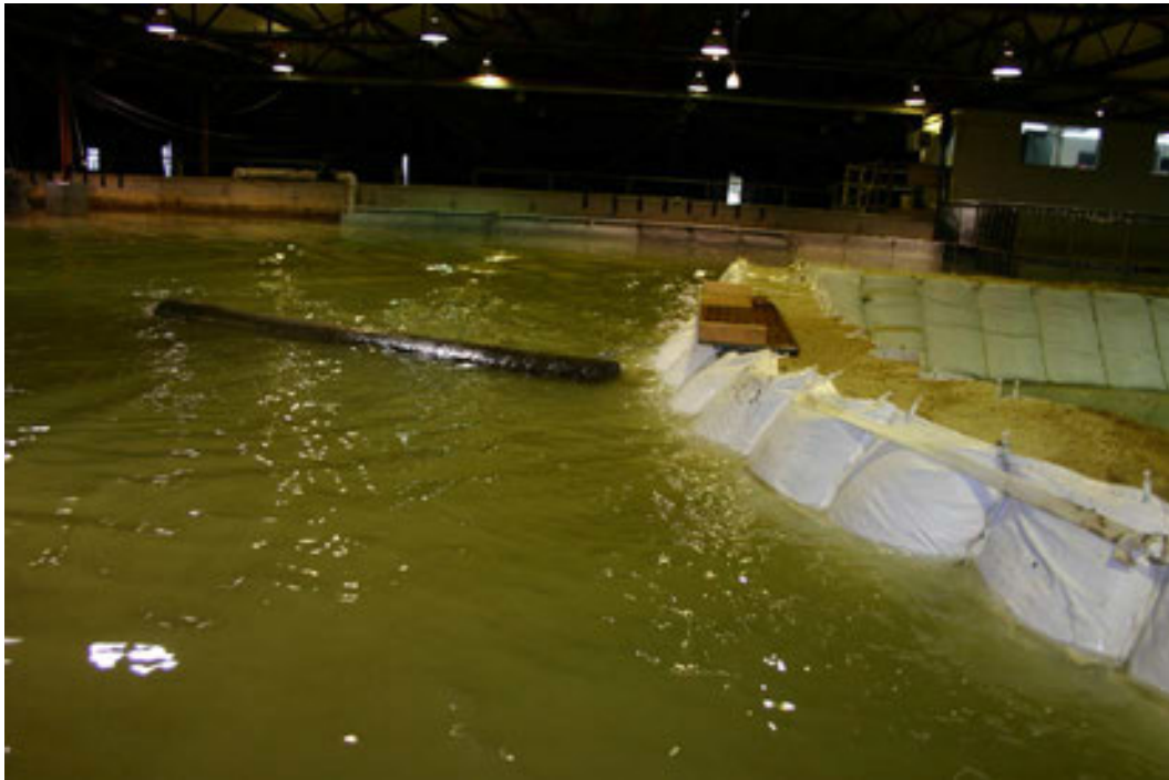
Figure 41. Immediately after log impact on barrier. The plywood on top of the barrier is to protect the barrier from the tow cable.
