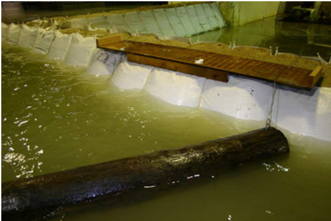
Figure 42. No damage to the barrier could be found.
