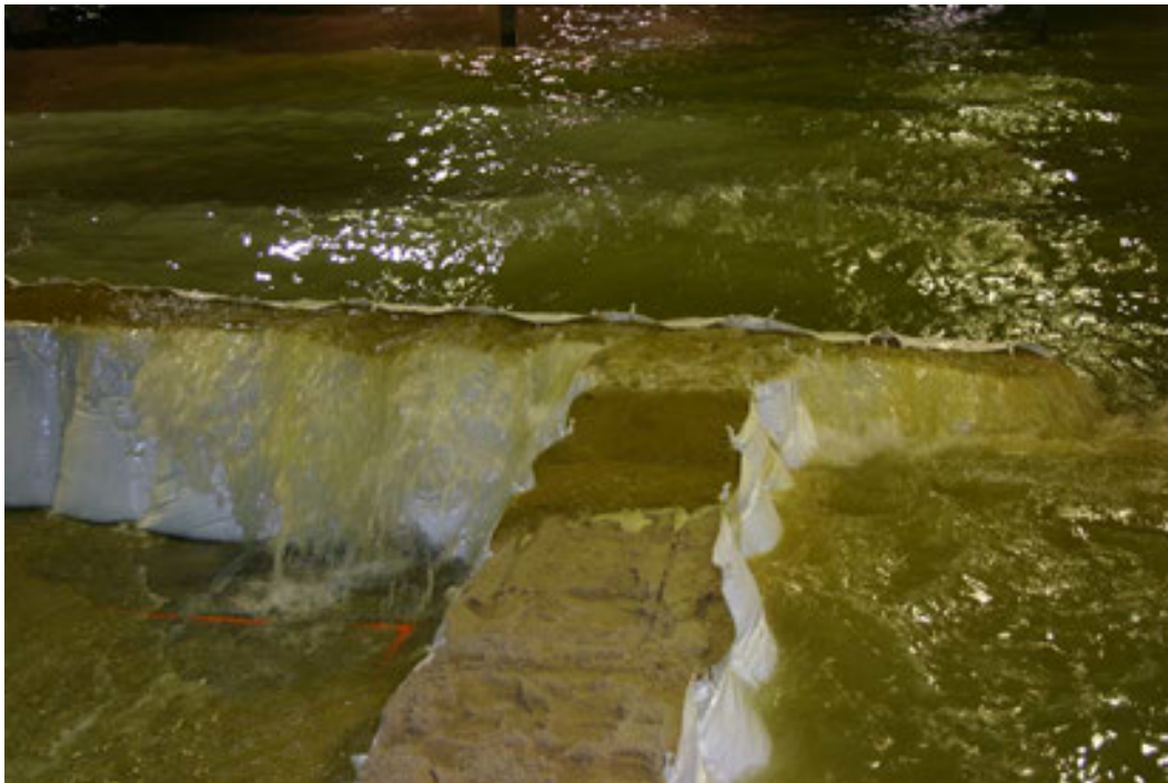
Figure 35. Overtopping along wall "B" during test with large waves at high water.
