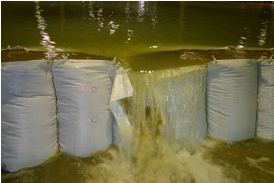
Figure 45. One bag cut open with water still overtopping structure.
